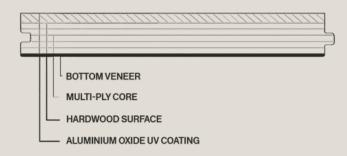
The Multi-Ply Core Structure Engineered Flooring is constructed with a crisscross arrangement that relieves internal stress and reduces the natural movement of timber. This results in a highly stable floor, allowing for cost-effective wide planks that are less prone to expansion and contraction.
