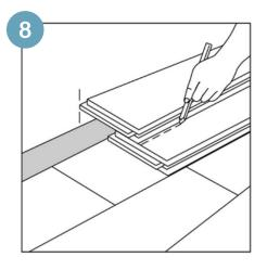
• To lay the last row: position a loose board exactly on top of the last row laid. Place another board on top, with the tongue side touching the wall. Draw a line along the edge of this boards, to mark the first board. Cut along the edge of this board to mark the first board. Cut along this line to obtain of the required width. Insert this cut board against the wall. The last row should be at least 50 mm (2") wide. The spacers can then be removed.
