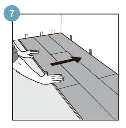
After 2-3 rows. Adjust the distance to the front wall by leaving an expansion gap of 10 mm (1/2").
