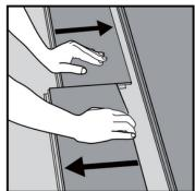
Separate the whole row by lifting it up delicately at an angle. To seperate the planks, leave them flat on the ground and slide them apart.
