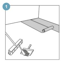
• After thoroughly cleaning the subfloor, you must install a foam underlay (unless your product has a pre-attached pad). Run the foam underlay in the same direction as the flooring planks. The underlay should be butted side-by-side with no overlap. Tape seams together. If you are installing over a concrete suboor, a 6-mil poly (plastic sheeting) is to be installed under the foam underlay. (Many foam underlays already have this plastic sheeting pre-attached).
