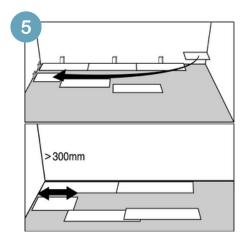
Start the second row with the leftover cut part of the last plank of the previous row. This small plank should measure at least 30cm (12").
