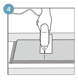
• If cutting with a jig saw, the laminate surface should be turned down. If cutting with a hand saw, the laminate surface should be face up.
