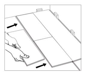
When installing each new row, take a full loose plank and use the long side to tap against the prior row to ensure no gapping.
