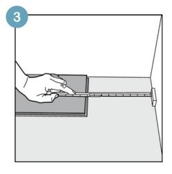
At the end of the first row, leave an expansion gap of 10mm (1/2") to the wall and measure the length of the last plank to fit.
