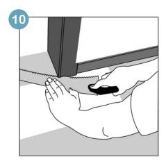
Door molding and skirting: lay a board (with the decorative side down) next to the door molding and as shown in the figure. Then slide the floorboard under molding.
