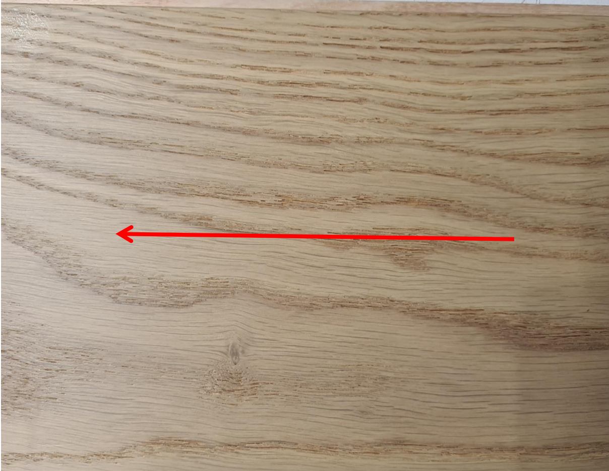
Figure 1: Castel Nuovo Collection Herringbone engineered timber plank Arrow indicates direction of testing
